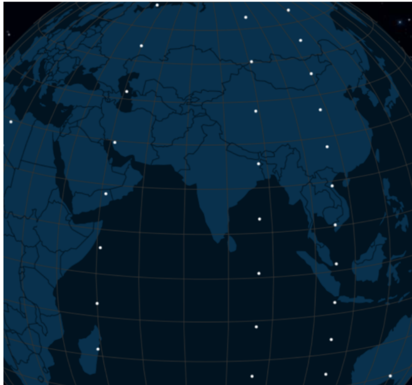
Figure 24. A segment of OneWeb's existing network showing its longitudinal orbit planes 157 .
